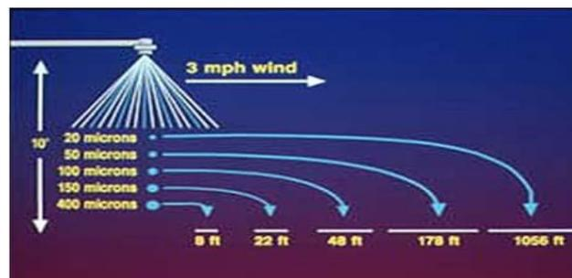
*Fig.5. Smaller droplets drift longer distances.*
